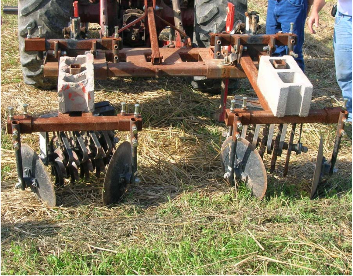
Figure 3. Two-row ripper and zone builder
