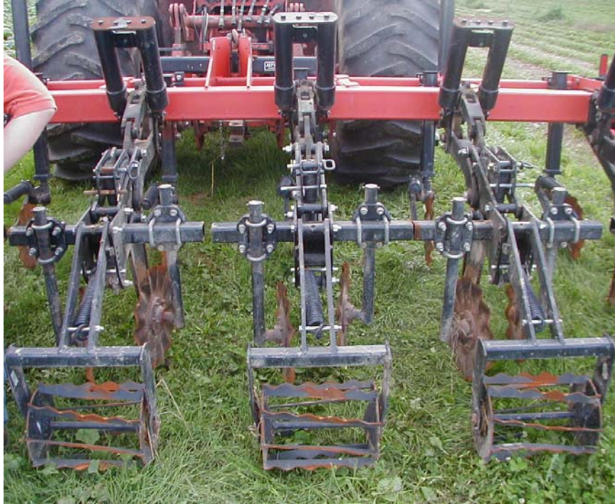
Figure 2. Hiller disks and rolling basket attachments
